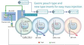
Inject eluate by setting the temperature of the injection port lower than the boiling point of the elution solvent and maintain as liquid in the
