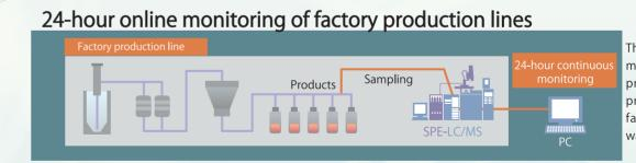
This system is effective for crisis management, such as checking products and products in each production line and process in factories, quality control, and wastewater check.
