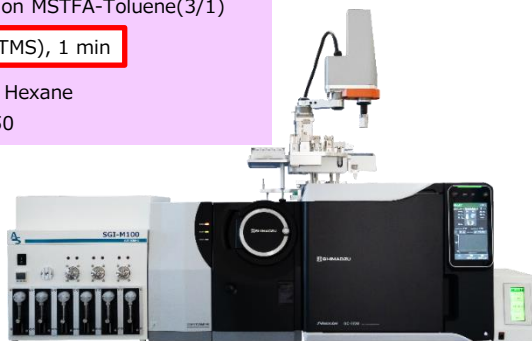
SPE-GC-MS system for metabolome analysis
