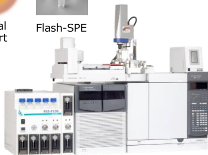
SPE-GC-MS system for metabolome analysis (Image)
