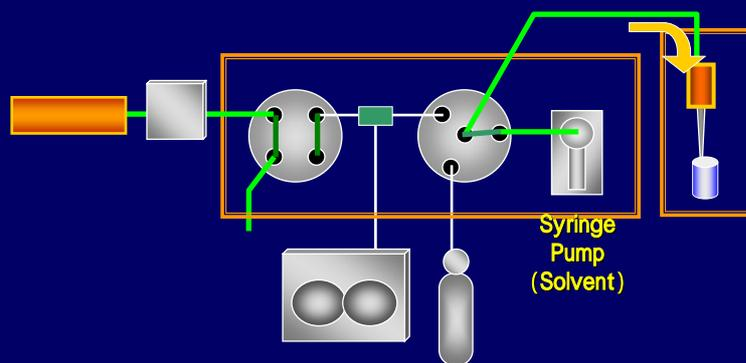
The SPE cartridge and tube are cleaned with a solvent.
