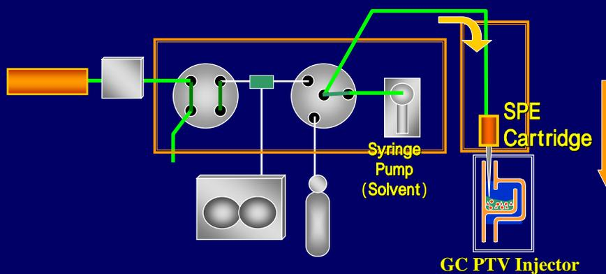
The target compound is eluted from the SPE with a solvent and the eluate is directly injected into GC injector via the injection needle.
