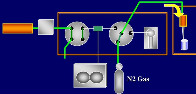
The SPE cartridge, tube and valve are dried with flowing nitrogen gas again.
