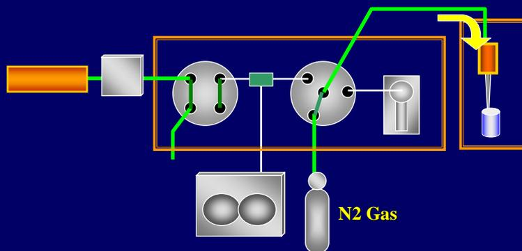
The SPE cartridge, the tube and the valve are dried by flowing nitrogen gas.
