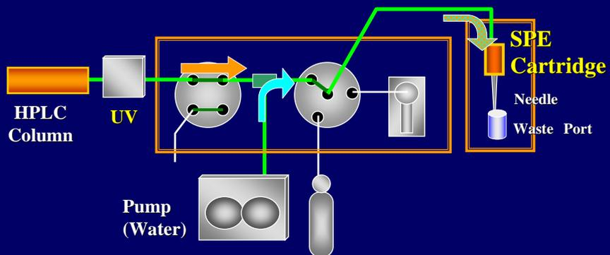
With adding water to the LC fraction, the diluted fraction is loaded on the SPE cartridge.
